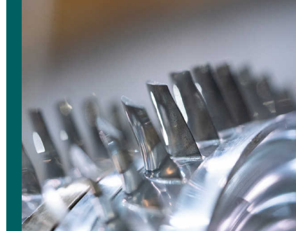
7HA gas turbine compressor.
